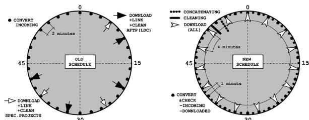
**Figure 1:** Old (left) and new (right) hourly schedule of basic action of NRT GOP data center.
