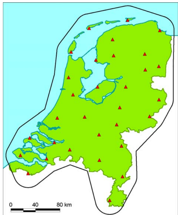
Fig. 1. 31 NETPOS reference stations (triangles) with an average distance of 40 km and the coverage (line) of the RTK service.
