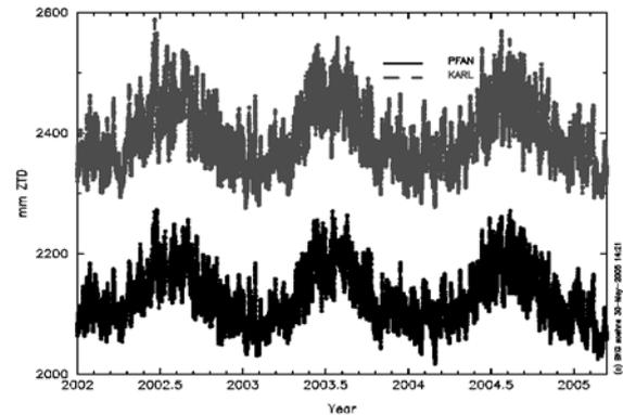
Fig. 1: Time series of Zenith Total Delay (ZTD) values for sites KARL and PFAN from EPN combined solution
