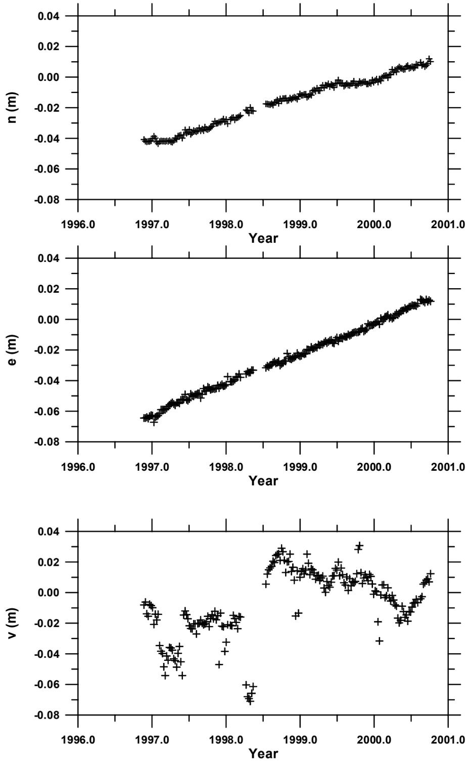
**Fig. 3.** Evolution of MOPI EUREF local coordinates in three components: north-south ( $n$ ), east-west ( $w$ ) and up ( $v$ ). The relative scale is given on the  $y$ -axes
