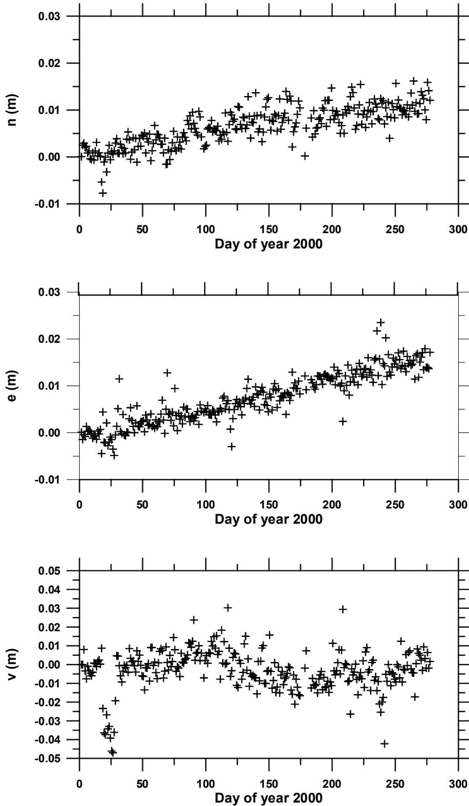
**Fig. 5.** Evolution of MOPI daily coordinates for GPS days 001-277 of 2000. Three components: north-south ( $n$ ), east-west ( $e$ ) and up ( $v$ ) are displayed. The relative scale is given on the y-axes.
