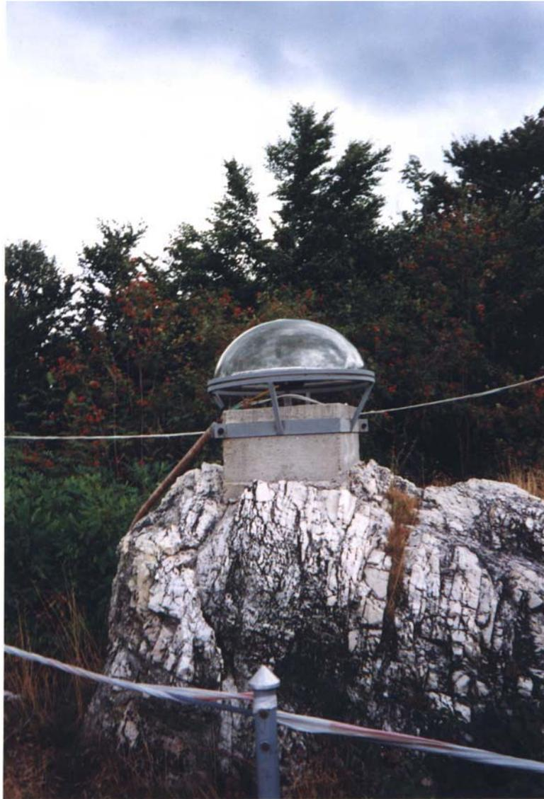
**Fig.1.** The concrete pillar for the GPS antenna with a radome for antenna protection
