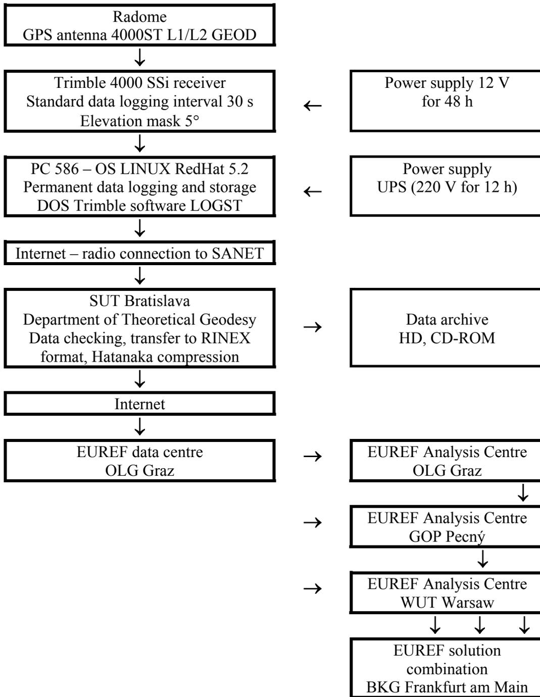
**Fig. 2.** Block diagram of hardware and software of MOPI permanent GPS station
