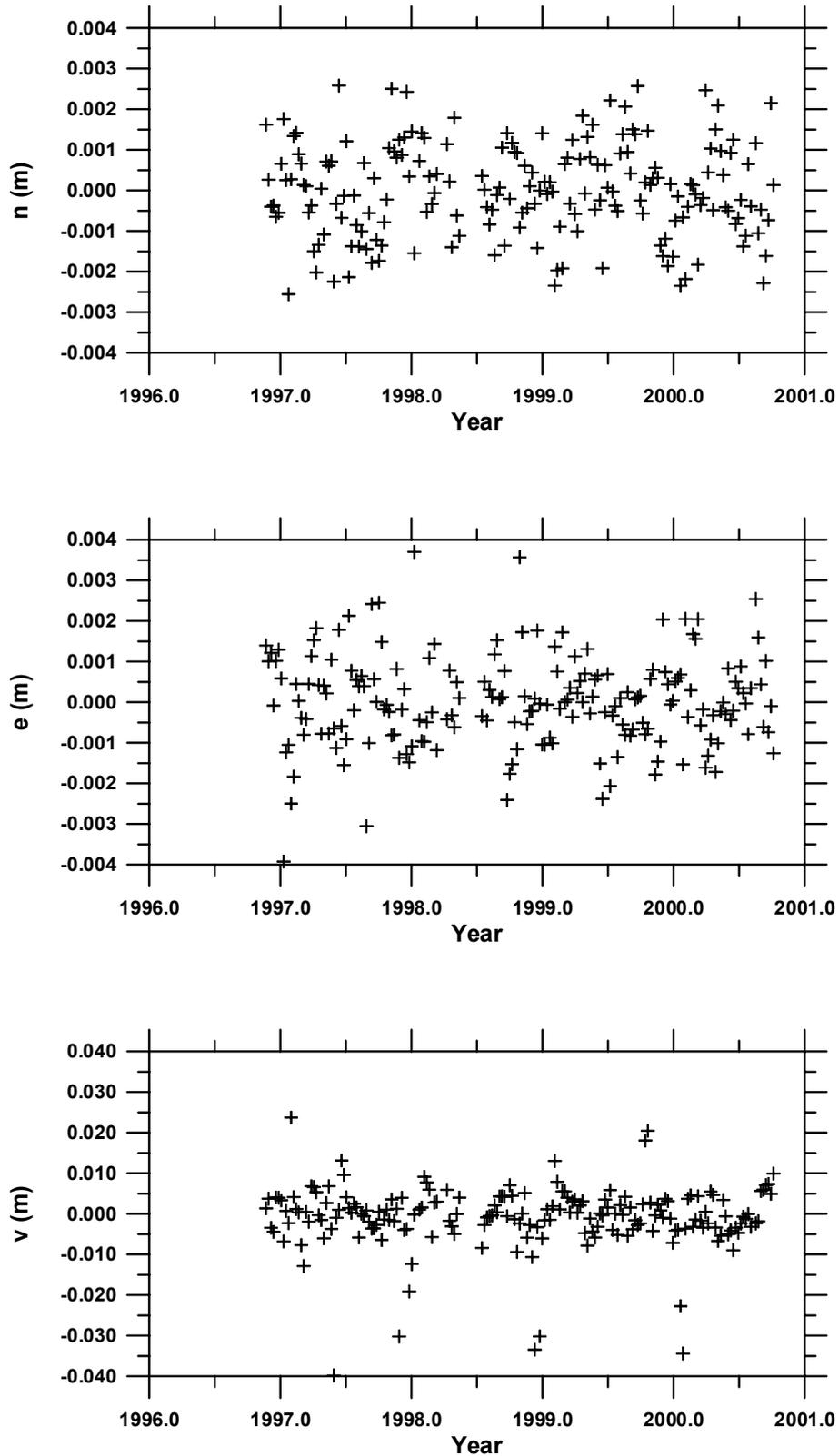
**Fig. 4.** Evolution of residuals from regression according to (1) in components: north-south ( $n$ ), east-west ( $e$ ) and up ( $v$ ).
