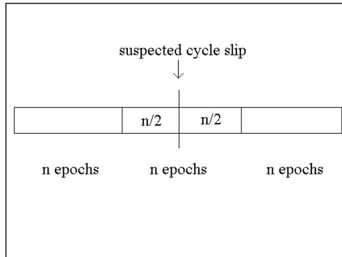
*Fig.2 - Sketch of cycle slip validation procedure*
