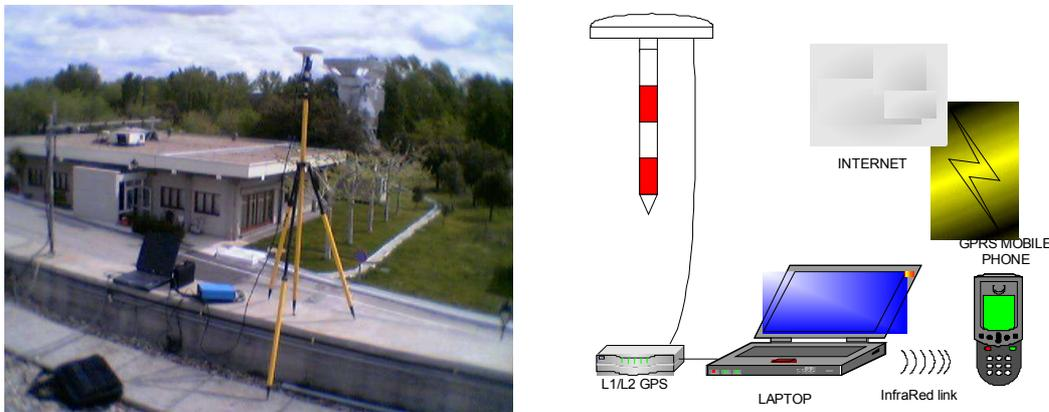
Figure 3: Bench mark Villafranca, 20 km distance from Madrid reference station (left), and General diagram of GPS rover configuration (right)
