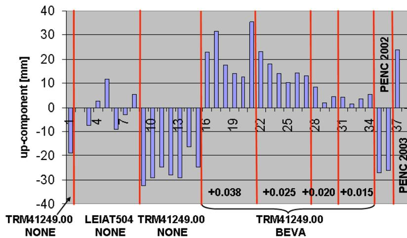
Fig. 6. Differences between TRM41249.00 antennas with radom BEVA and without to LEIAT504 antennas. Variations when the antenna height within the BEVA radom changes. Changes of PENC-WIEB after the jump of PENC (2003). Always phase corrections IGS/NGS used.
