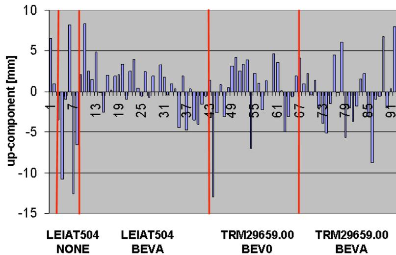
Fig. 5. Differences between TRM29659.00 with radoms BEVA/BEV0 and LEIAT504 antennas.
