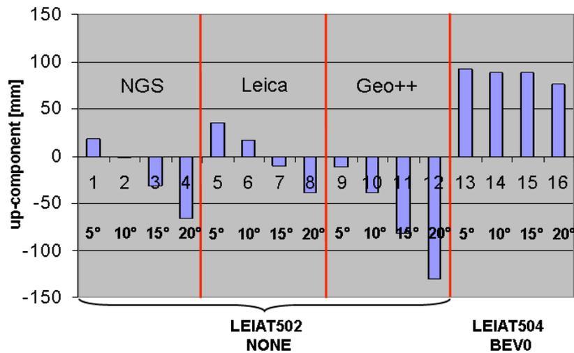
Fig. 9. Differences between LEIAT502 antennas and LEIAT504 antennas. Different phase correction sets of NGS, Leica and Geo++ are used.
