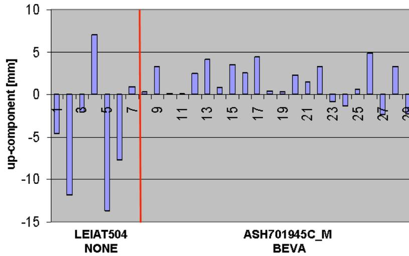
Fig. 4. Differences of ASH701945C\_M with radom BEVA to LEIAT504 antennas.
