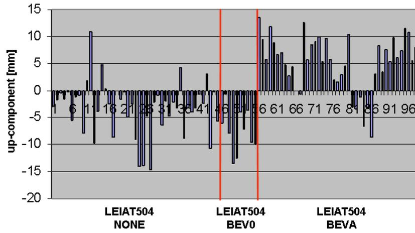
Fig. 3. Differences of LEIAT504 antennas with different radoms.
